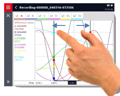
Fig.: Using the magnifying gesture with two fingers, the operation is carried out - Zooming in this case.
