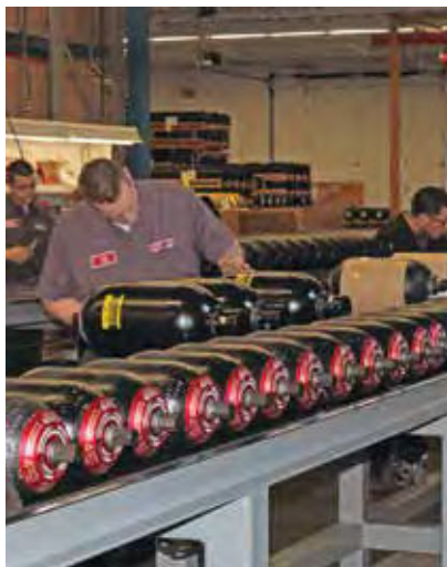
Bladder Accumulator Assembly Area
