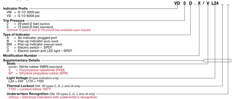
W = "VD..." indicator modified with a brass piston for use with High water based emulsions/solutions (HFA) & (HFC) (For additional details and options, see Section G - Clogging Indicators of the HYDAC Filter catalog.)
