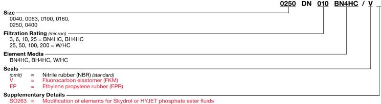
Modication of "V" elements for use with oil water emulsions (HFA) and water polymer solutions (HFC) usually polyglycol
