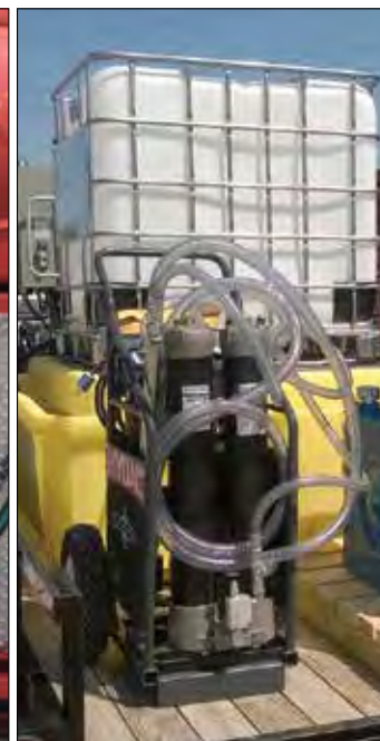
OFS Filtration Station with HPU.
