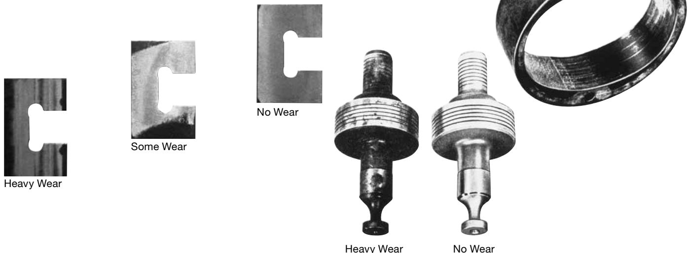
Figure 1. Typical Examples of Wear Due to Contamination
