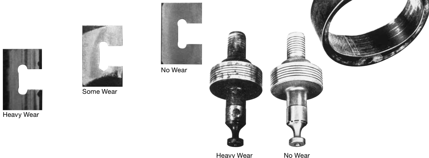
Figure 1. Typical Examples of Wear Due to Contamination
