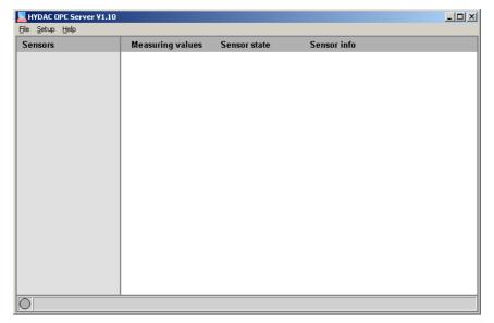
You can use the menu item SETUP -> CONNECTIONS in the main menu of the program to establish the connection to the individual sensors. The devices/sensors are added to a list. This list is saved by confirming with the OK key. The online measurement is then started.
