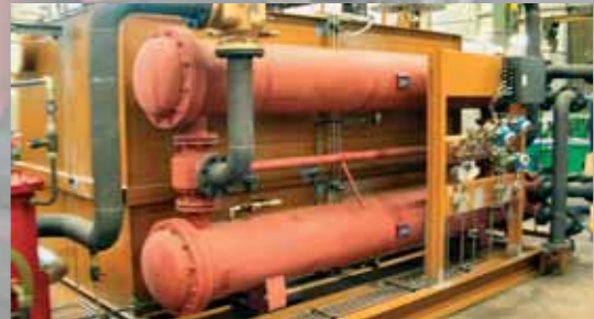
Blast Furnace Gas Expansion Turbine, oil tank volume 9,500 l, power 500 kW, flow rate 760 l/min.
