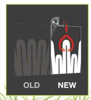
Under high dynamic load conditions, the Helios geometry prevents pleat compression which reduces differential pressure.
