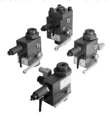
The fluid side has to be protected against excessive pressures with approved safety valves. HYDAC provides the pressure relief valve (*DB12 Series*) which has a pressure setting (*set by HYDAC*) up to 5800 psi (400 bar). The sealed valves carry a CE mark, and are integrated into the Safety and Shut-off Blocks in nominal sizes DN10 to DN32
