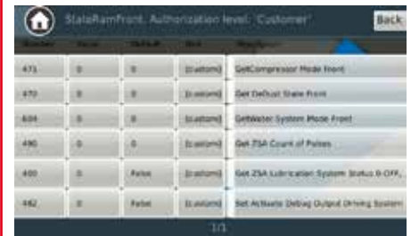
Parameterisation using the Service Tool functionality on the display
