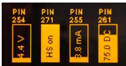
The image shows the integrated OLED display, e.g. to indicate test settings, pin numbers and equipment IDs
