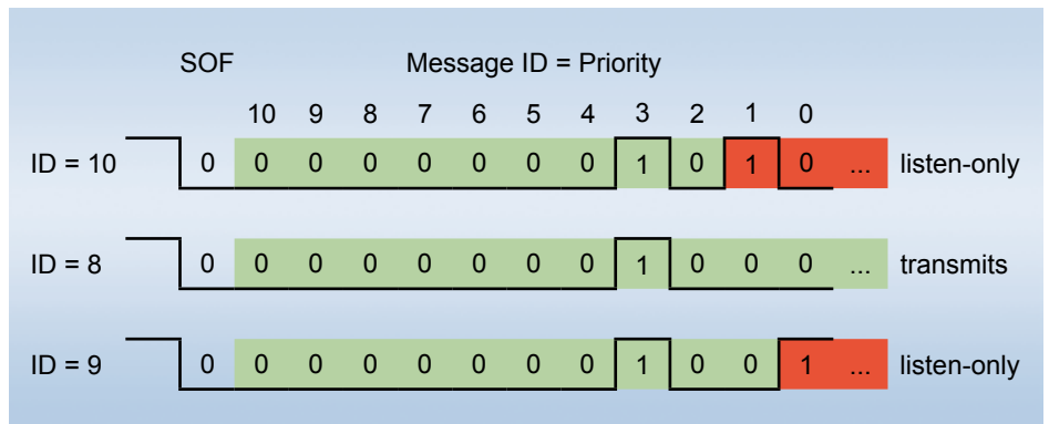
Figure 13: Arbitration of transmission rights
