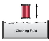
1. Remove external build-up of contamination with cleaning fluid in separate tank.
